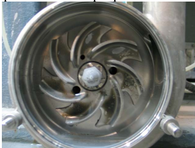
Figure 10 - New Improved Off-Gas Pump Impeller at the End of the Long Duration
