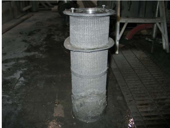
Figure 12 - Basket Condition at the End of 10 Weeks of Testing
