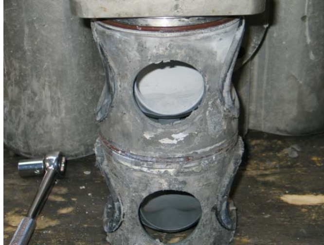
Figure 11 – Suction Strainer Internal Mechanism at the End of the Long Duration
