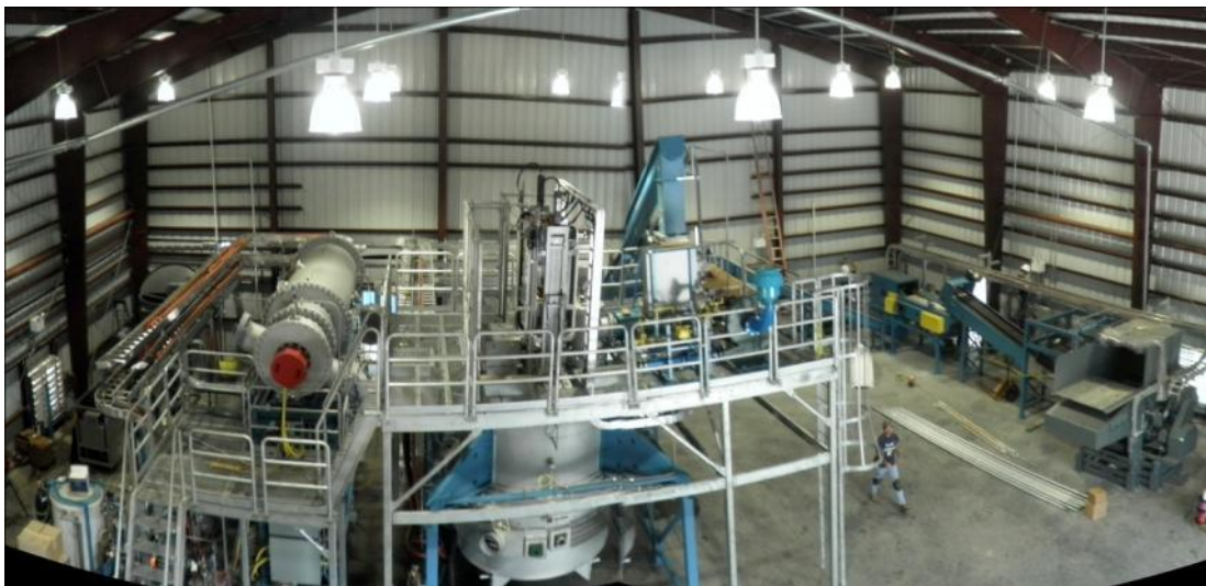
Figure 4. 10.5 TPD PRR system – Thermal Section
