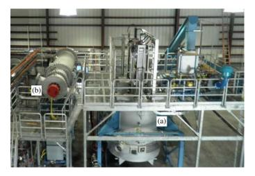
Fig. 2. (a) Picture of the arc furnace and (b) secondary gasification chamber of the 10.5-ton-per-day PRRS facility in operation at the Hurlburt Field U.S. Air Force facility.
