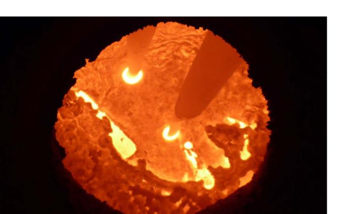
Fig. 3. Picture of the arc furnace in operation, showing two graphite electrodes driving an electric arc through slagged inorganic material and gasifying organic waste.
