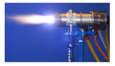
Fig. 1. Picture of the air plasma torch used in the secondary gasification chamber to refine the syngas produced in the arc furnace.
