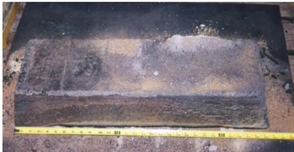
Fig. 4. Vitrified block of Hog fuel boiler ash.
