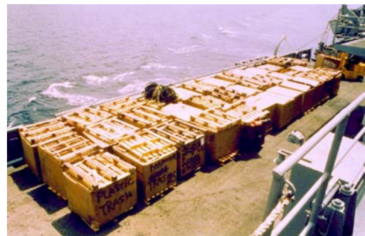
Fig. 1. Triwall boxes containing the average amount of solid waste generated daily by a Nimitz class aircraft carrier.
