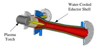
Fig. 2. Schematic of Plasma-Fired Eductor
