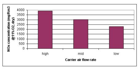
Fig. 7. Effect of Reducing Carrier Air Flow on NO<sub>x</sub> Emission
