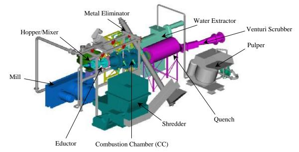
Fig. 1. Overall Layout Drawing of PAWDS
