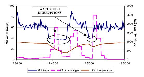
Fig. 5. Example of Data Acquisition During Inconsistent Feed Periods
