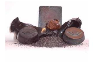
Fig. 3. Sample Products from Slag
