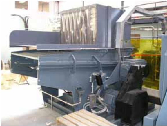
Figure 2 Example of a Shredder Used on the Marine System
