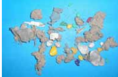
Fig. 7. Poorly Milled Plastics
