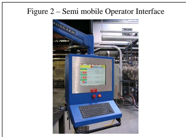
The control program is designed with two levels of accessibility: the operator level and the supervisor/maintainer level, which is password protected.
