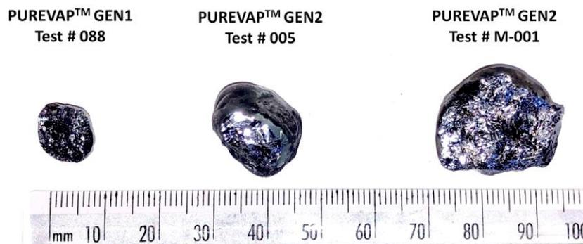
Picture 1. Largest Individual Silicon Nuggets per testing stage on the left with GEN1, in the middle with GEN2 and on the right with GEN2 after modification
