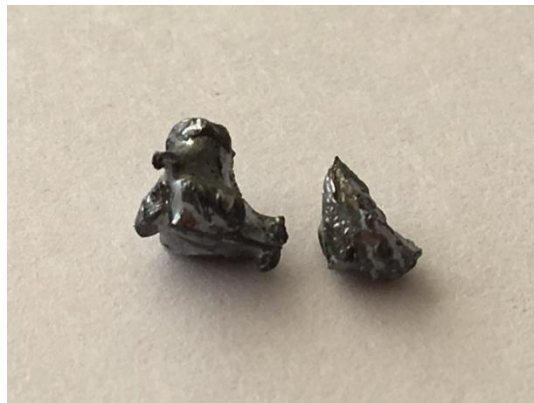
First nuggets of silicon metal produced during test #15
