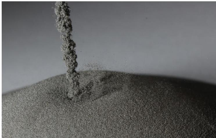
Figure 1. PyroGenesis' Ti-6Al-4V powders
