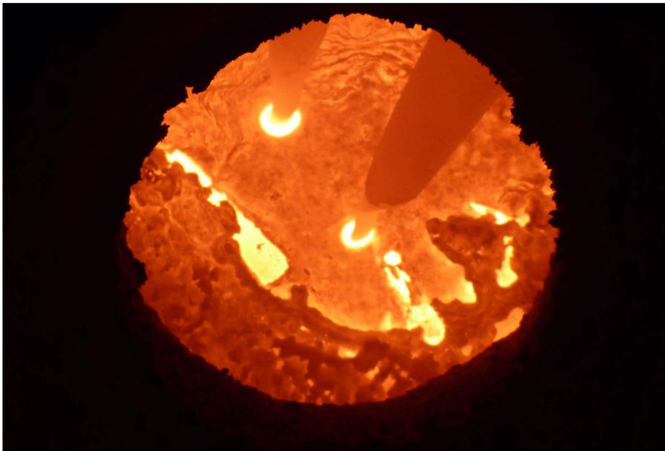
Fig. 3. Picture of the arc furnace in operation, showing two graphite electrodes driving an electric arc through slagged inorganic material and gasifying organic waste.
