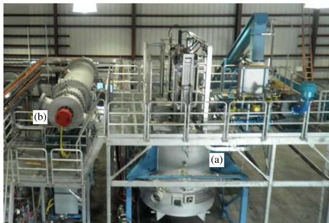
Fig. 2. (a) Picture of the arc furnace and (b) secondary gasification chamber of the 10.5-ton-per-day PRRS facility in operation at the Hurlburt Field U.S. Air Force facility.
